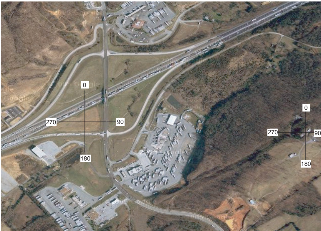
FIGURE 1 Site map at I-40 and Watt Road showing locations of monitoring sites, Interstate, and nearby truck travel centers (scale: monitoring sites are 3,300 ft apart).
