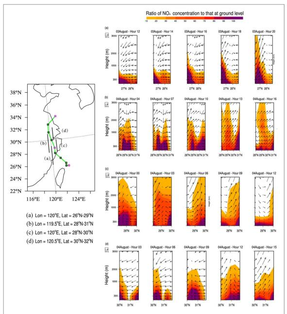
**Figure 2.** Latitude–height cross sections of the ratio of the NO<sub>x</sub> concentration to that at ground level with the vertical wind vector superimposed at (a) 120°E, 26°N–29°N, (b) 119.5°E, 28°–31°N, (c) 120°E, 28°–30°N, and (d) 120.5°E, 30°–32°N. Note that the pink boxes in the left inset represent typhoon locations at 00:00 UTC, while the black ones represent the typhoon locations every 6 h.
