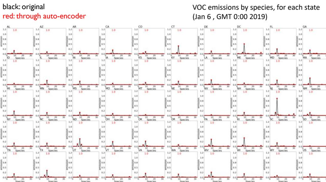
(b) performance in decoding the VOC emission profile by states (using 2 latent variables to represent the original 33 VOCs, the red number represents the  $R^2$ )
